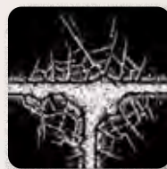
8 Cracked "T" Passages
